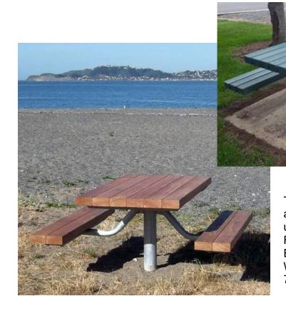
The Peninsular Picnic Setting above is installed in Te Aroha and uses long-lasting 90 x 65mm Replas recycled-plastic slats. In Eastbourne on the shores of, Wellington Harbour, 145mm x 70mm hardwood slats were fitted.
